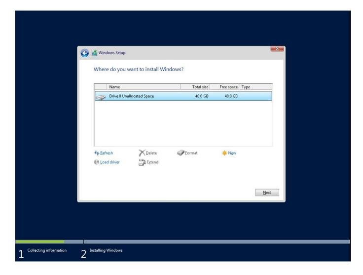
8. Setup automatically creates a new partition filling the entire disk space. Alternatively you could have selected "New" at the previous step to create a disk partition sized to your requirement.
